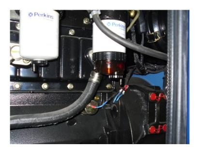
The fluid in the bottom of the diesel filter should be reddish in colour, if there is a clear liquid under the reddish diesel this indicates water is in the fuel and the water should be drained off using the drain tap under the filter.
