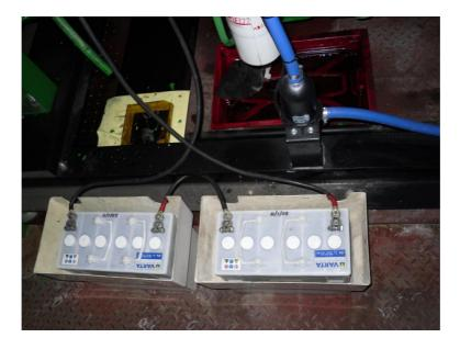
Further along are the main batteries shown above with their protective top cover removed, these are checked in exactly the same way as the spare standby batteries in the step carried out previously (electrolyte level checking and toping up)
