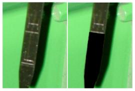
The picture on the left above shows the dipstick dry to show the markings, the High and Low marks are clearly visible, the oil level upon removal of the dipstick should be between the 2 marks but near the high mark as much as possible. The right picture shows the oil level at its correct position. The oil should look a golden brown to black colour. If the oil has a white milky look or anything different then this could indicate an internal engine problem and Dale Power should be consulted.
